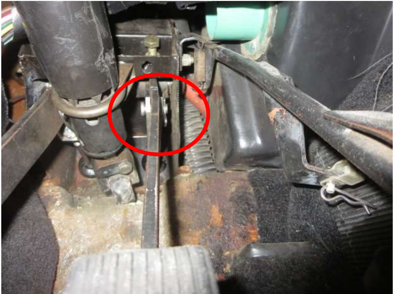
Figure 3 brake clevis pin and hitchpin
