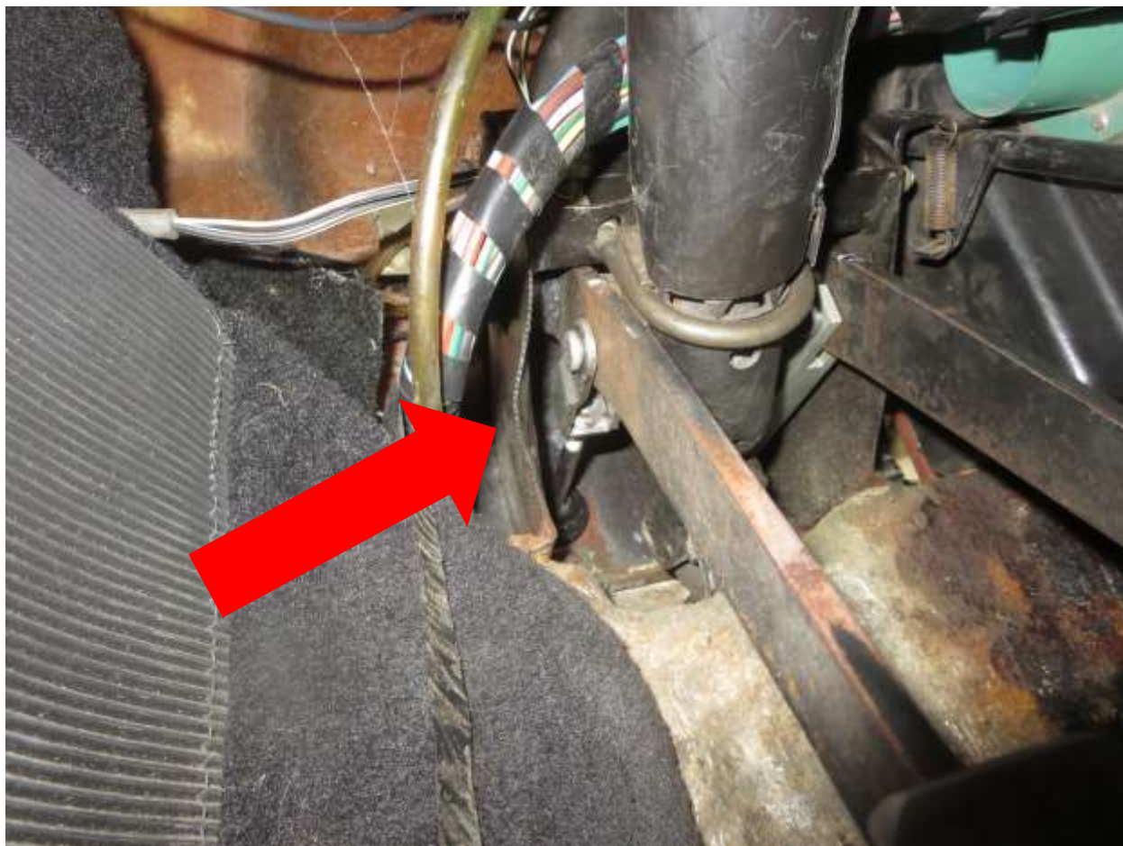
Figure 4 Clutch clevis pin and hitchpin. Note bent pedal box for clearance
