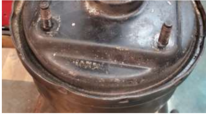
Figure 7 Crimped edge on Esprit servo
